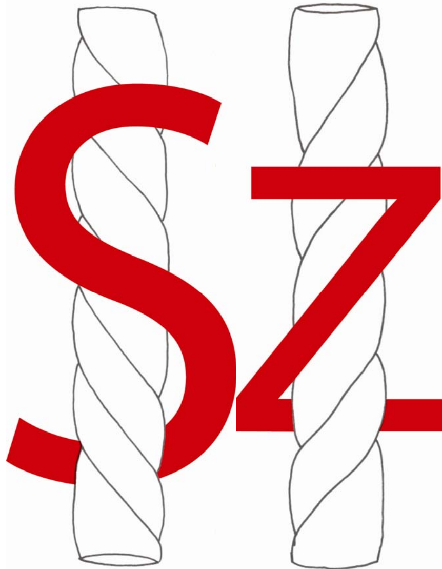
Figure 4-2: Determination of S-twist and Z-twist for a cord
