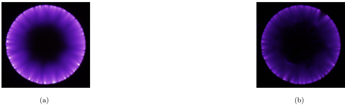
Figure 7.4: Photographs showing the effect of seeding contamination on the plasma before (a) and after (b) a quiescent flow PIV run.
