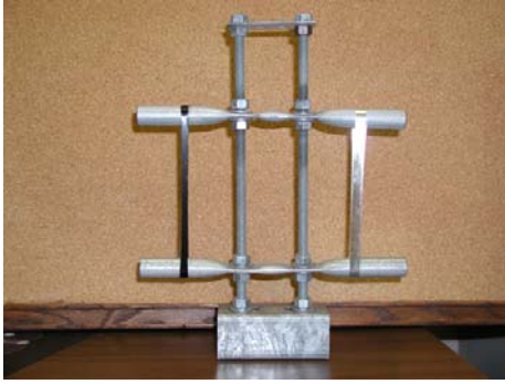
Figure 2-2 Constant length stabilization rack
