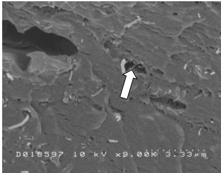
Figure 3-11 Craze bridging of MWNT
