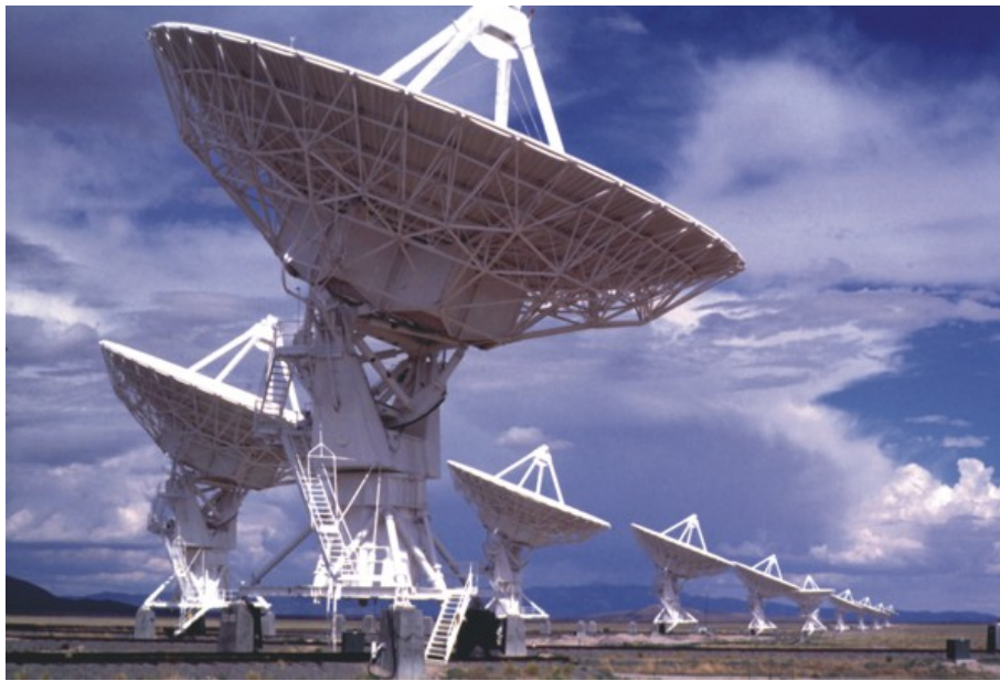
Figure 1.3: The Very Large Array (VLA) radio telescope in Socorro, New Mexico, is a connected-element radio interferometer that consists of 27 antennas each with 25 m diameter. The images show the VLA at its most compact configuration (D Array), which has a maximum antenna separation of 1 km. The extended configuration of the VLA, known as A array, has a maximum antenna separation of 36 km, corresponding to an angular resolution of 50 mas at 43 GHz. Image courtesy of NRAO/AUI.
