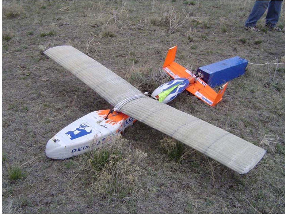
Figure 3.4: Recovery of second-generation inflatable-rigidizable high-altitude test article.
