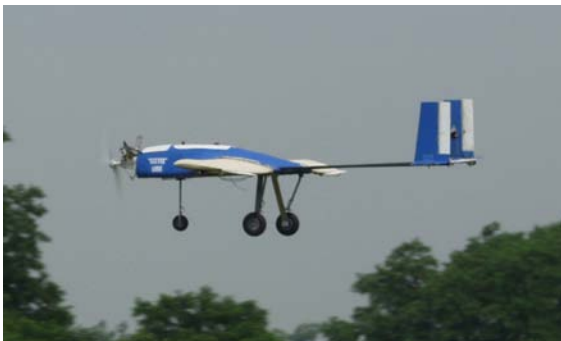
Figure 7.18: Flight test with Vectran wings on AIRCAT.
