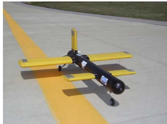
(b) ILC Dovers multi-spar nylon inflated wing on flight test vehicle.
