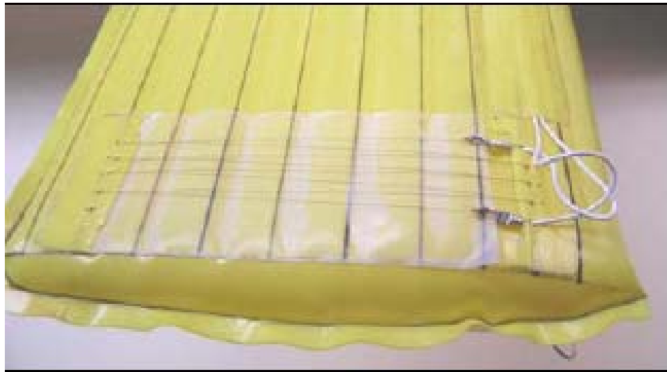
Figure 5.24: SMA wires integrated to an inflatable wing.
