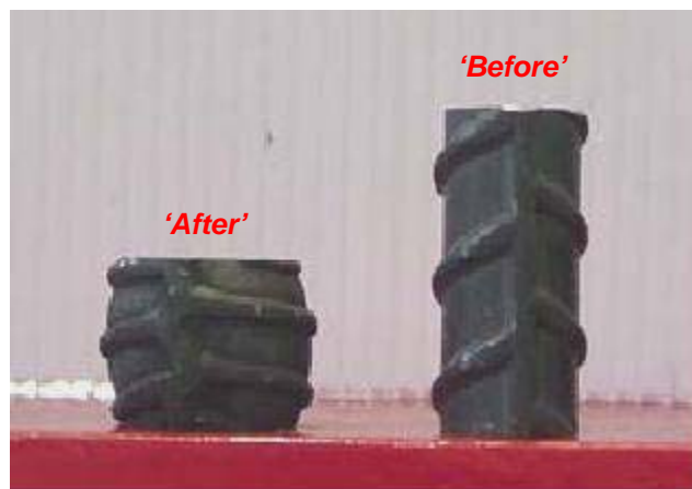
Fig. 2.14 – Compression failure of short steel specimens (El-Hacha and Rizkalla 2002).
