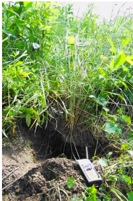
Picture 5.9. A soil pipe opened through exfiltration pressure in the grass approximately 12 m above the head of a major gully following large rain events in May. A large animal burrow was most likely utilized for emergence. Photo by author, May 2004.
