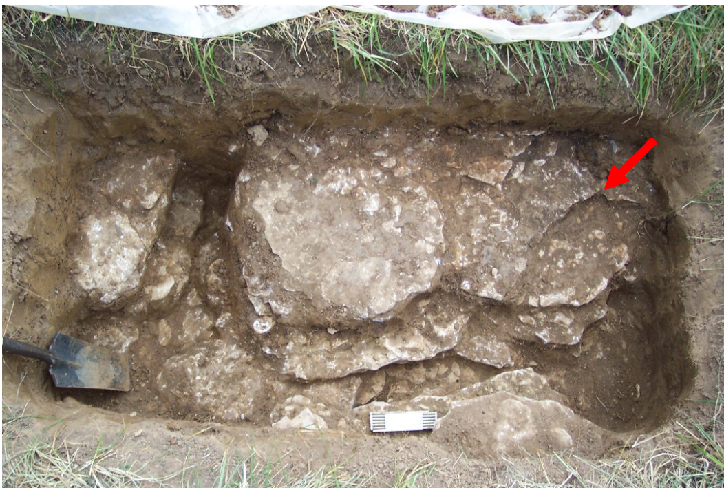
Figure 5.40. Bedrock plates under grass display a roughened, subangular surface in pit 13. Stones are rounded where weathering has attacked corners. Red arrow shows the location of a sharp edge where a tight-fitting plate was removed along an unweathered fracture. Photo by author, September 14, 2005.
