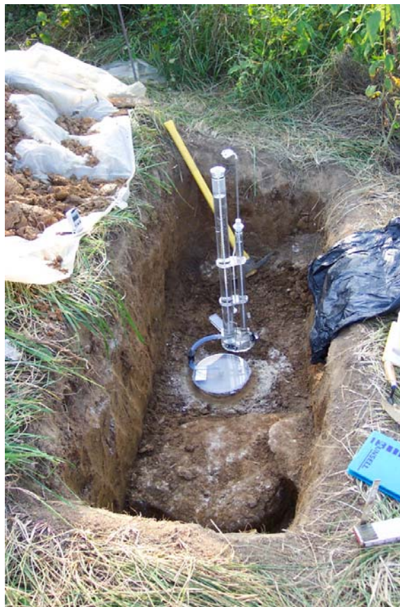
Figure 6.3. Pit 14 infiltration tests at 55 cm were taken less than 15 cm above bedrock in soil found to be 60% clay with few to common fine roots between the disk and the root mat on the rock face. Near-saturation K(-3) calculated for this spot was 2.48 \text{ cm hr}^{-1} , which almost equals the conductivity calculated for the deep-soiled, much more organic and pore rich sink location shown in Figure 6.2. Photo by author, July 2005.
