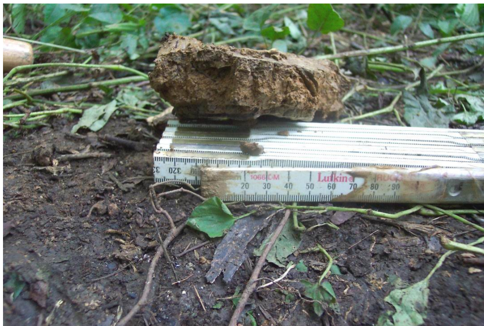
Figure 5.33. Soil discoloration from contact with limestone plates at the bottom of forest pit 5. Photo by author, July 22, 2005.
