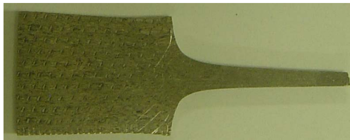
Figure 4.4: Material flow from the grip region into the gauge length region
