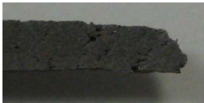
Figure 6.5: Evident cavitation in a specimen deformed at 400 °C and 5 \times 10^{-5} \text{ s}^{-1}
