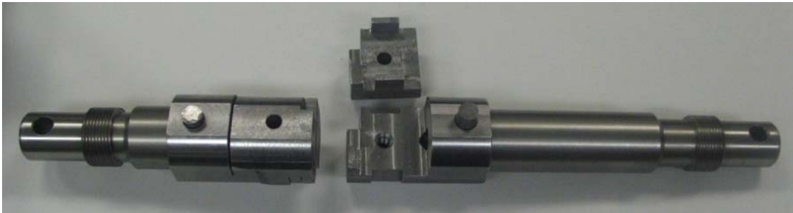
Figure 4.8: Type-II grips for high temperature tensile testing (for post-SPF in particular)
