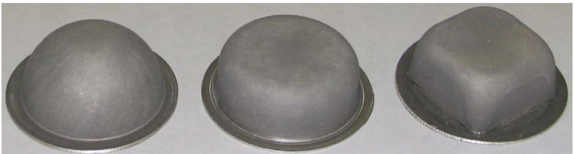
Figure 4.17: Examples for magnesium sheets formed into different shapes using type-I forming dies
