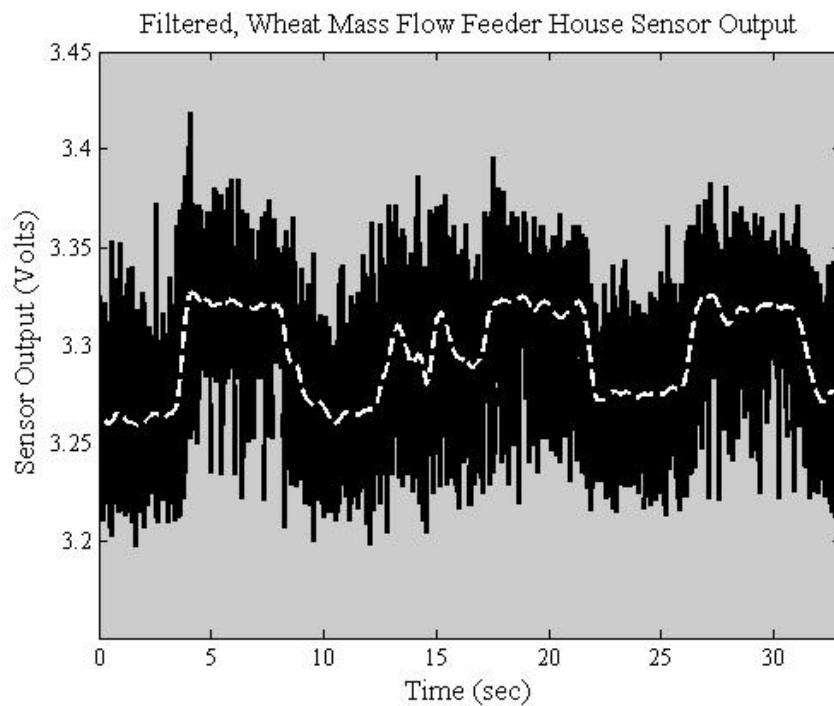
Figure 3.19. Filtered feeder house sensor output under ASABE X579 wheat mass flow conditions.
