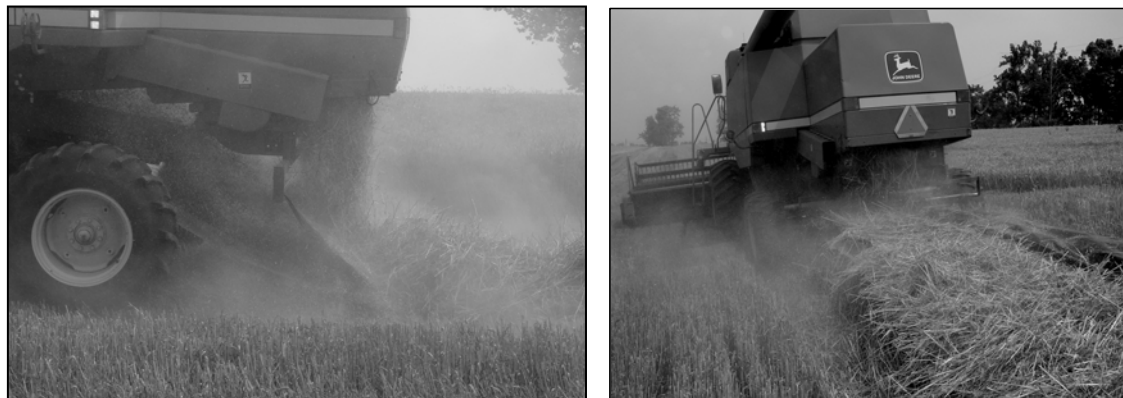
Figure 3.4. Obtaining Material Other than Grain (MOG) samples during the 2005 summer wheat harvest to determine the volume of material fed through the combine.
