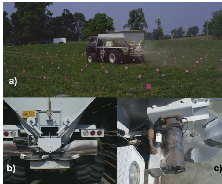
Figure 5.1. Newton Crouch spinner disc applicator; a) isometric view of applicator b) rear view showing spinner discs, and c) hydraulic drive motor and source fluid power control valve for apron chain.
