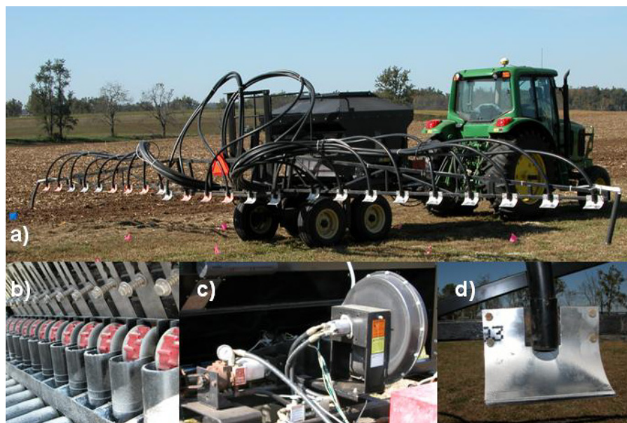
Figure 5.3. Gandy Orbit-Air pneumatic applicator; a) isometric view of applicator b) fluted metering rollers, c) centrifugal blower and Rawson hydraulic control system, and d) deflector plates.
