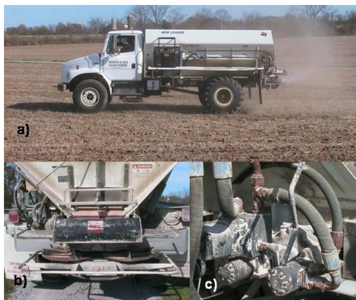
Figure 5.2. New Leader L3020G spinner disc applicator a) side view of applicator b) rear view showing spinner discs, and c) hydraulic drive motor and control valve for apron belt.
