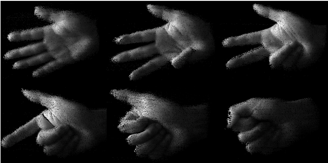
Figure 2.4: Sample point clouds, using PMP with N = 4 , live show of various hand poses.
