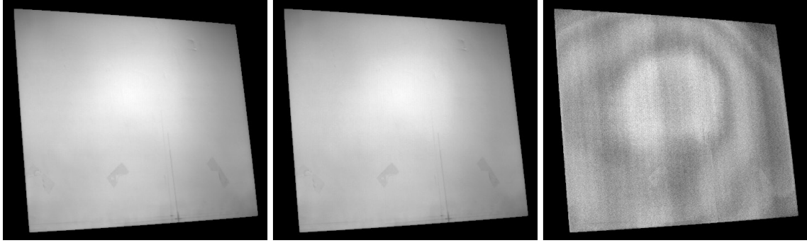
Figure 1.44: The visualization of magnitude of harmonics: (left) first order, (middle) second order, and (right) third order.
