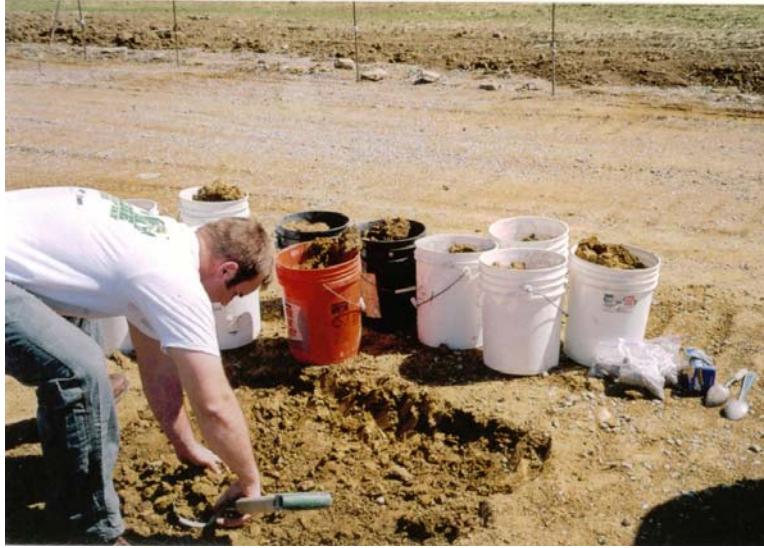
Figure 5.4 Soil Excavated Approximately 6 inches – 1 foot Deep.
