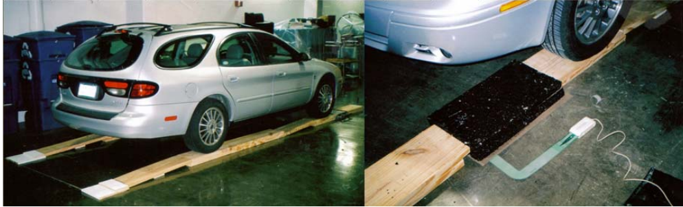
Figure 4.6 Car on Ramps Leading up to Portable Scales (left) and Tekscan Sensor Install Between Asphalt Layers (right).
