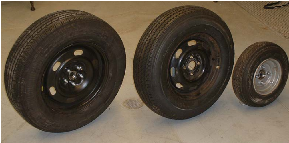
Figure 5.10 Radial Tire (Left), Bias Ply Tire (Middle), Small Utility Trailer Tire (Right).
