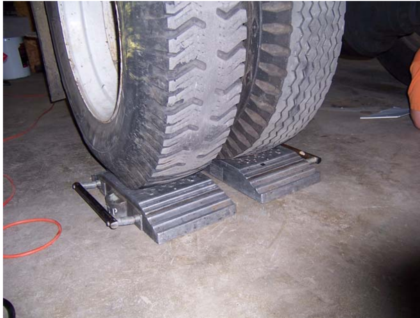
Figure 4.5 Portable scales used to measure wheel load for calibration.
