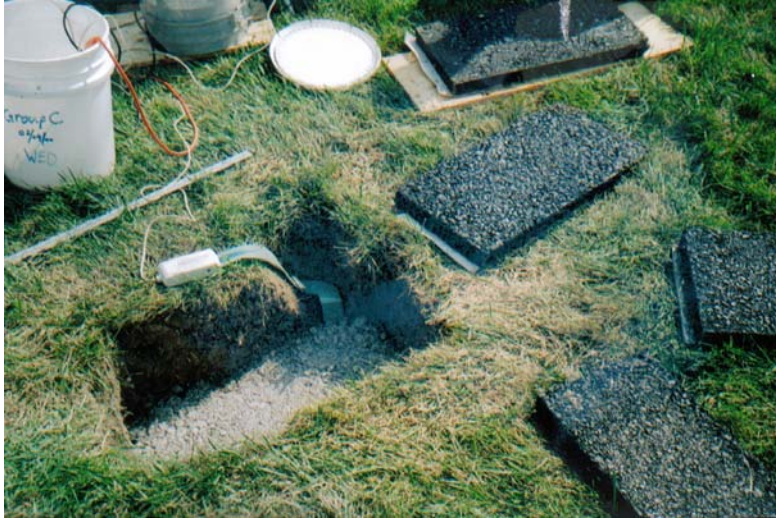
Figure 4.8 Tekscan Sensor Installed in the Test Hole.
