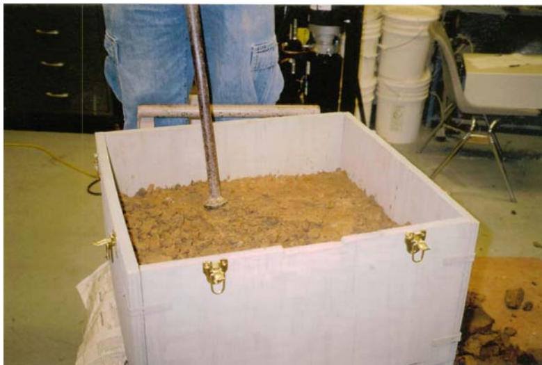
Figure 5.5 Compacting Clay with Iron Digger.
