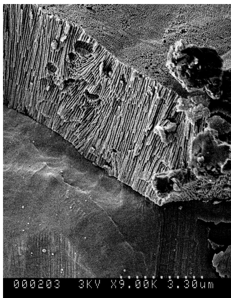
Figure 4.20 SEM of cross-section of porous alumina foil – low magnification
