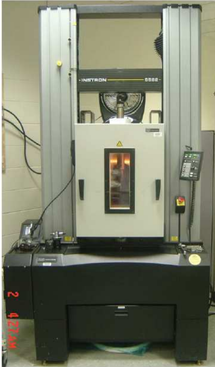
Figure 12 : Load Frame equipped with a chamber [Abu-Farha, F., 2007]
