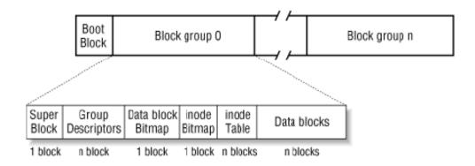
Figure 4.3: Layout of an Ext2 partition
