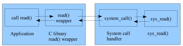
Figure 4.1: Invoking a system call.
