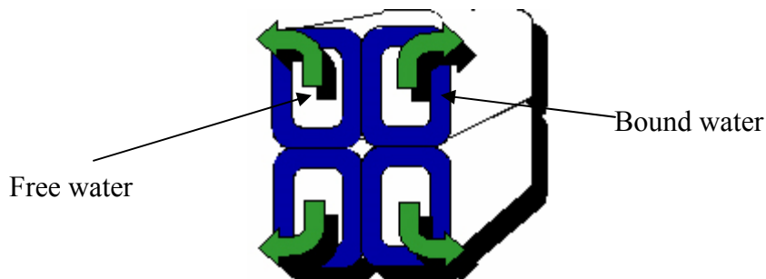
Figure 1-2: Section of wood cell showing the drying of free water.
