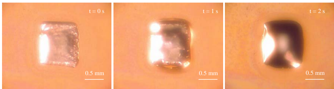
Fig. 6.18 Extracted images representing the sequence of spreading of eutectic Sn-Cu solder alloy on a highly polished surface (Met. lab)
