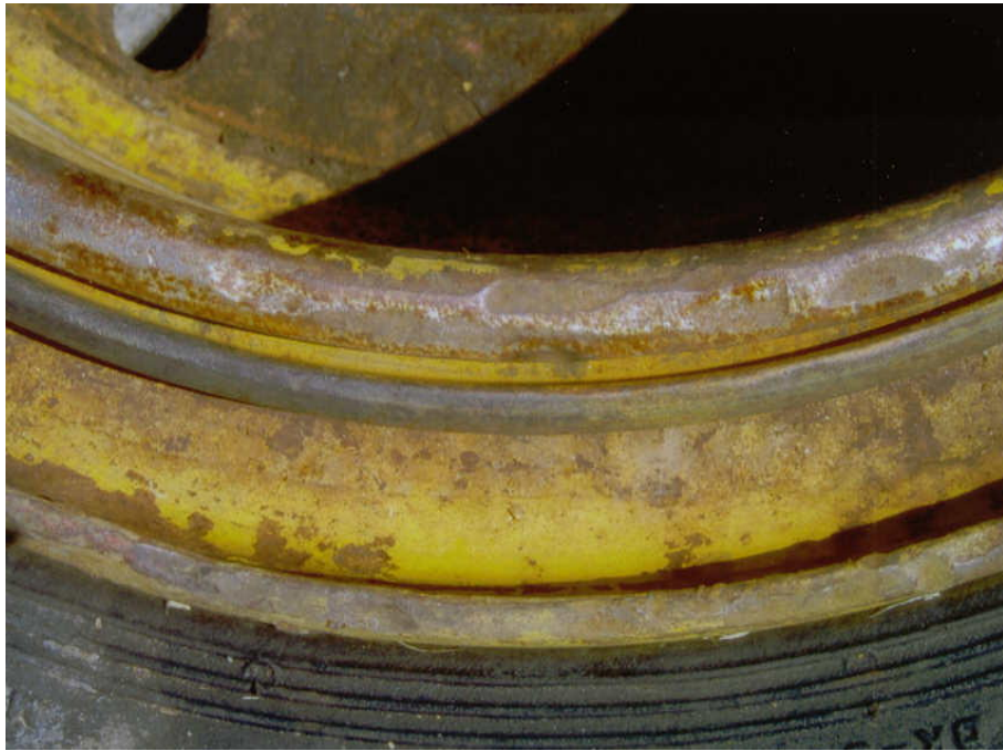
Figure 3.12: Rotational dislocation of ring portion from rim base at position 2.
