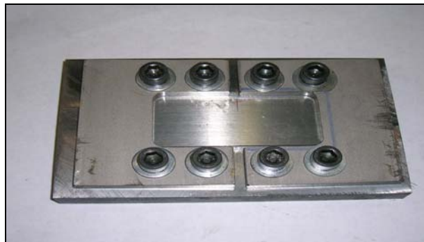
Figure 3- 2 Assembly of backing plate holding plates and sample
