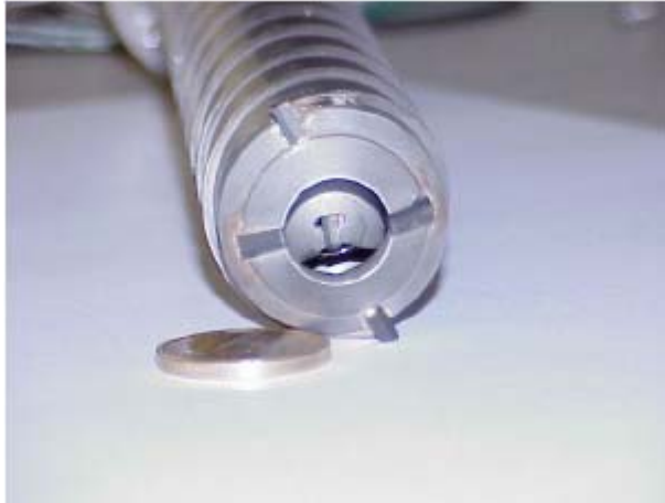
Figure 2.1: DeeDri PCD compact core drill along with sampling mechanism developed by the Italian space agency (Magnani et al., 2004)
