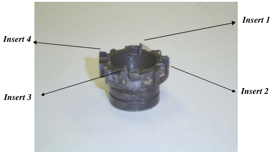
Figure 3.1: PCD compact core drill showing the four inserts
