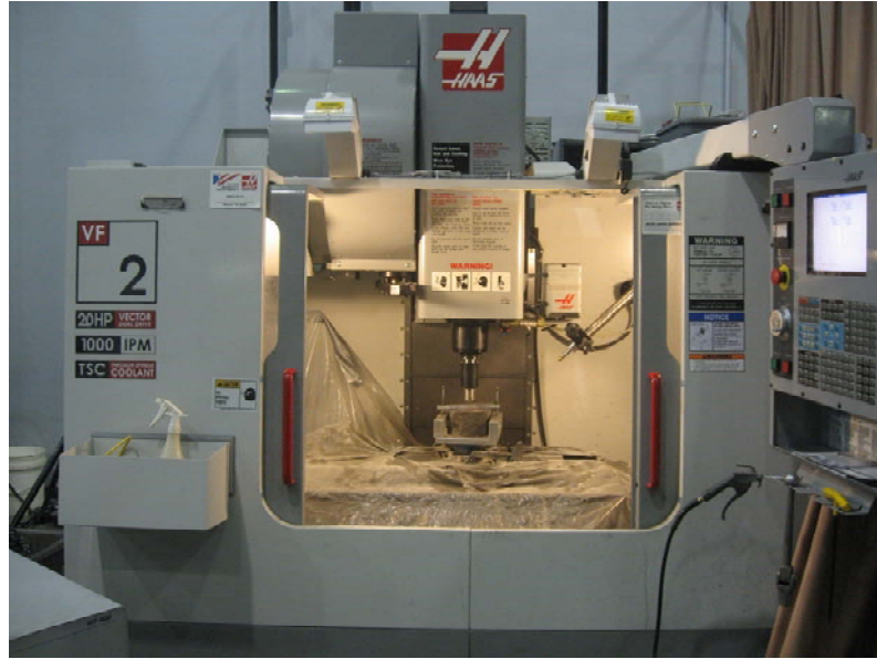
Figure 3.3: Experimental set-up for core drilling of basalt at University of Kentucky Machining Research Laboratory
