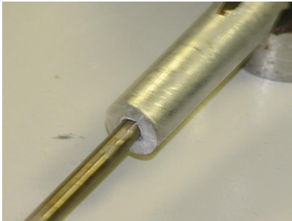
Figure 53 Photo of the bolt electric resistance heater capable of 450°C
