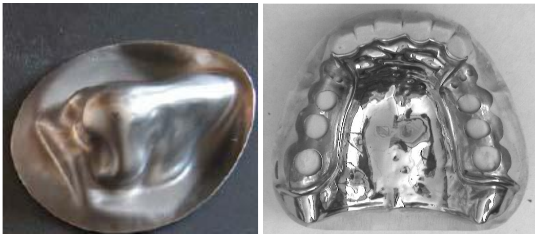
Figure 7 Superplastic forming used for medical applications (3)
