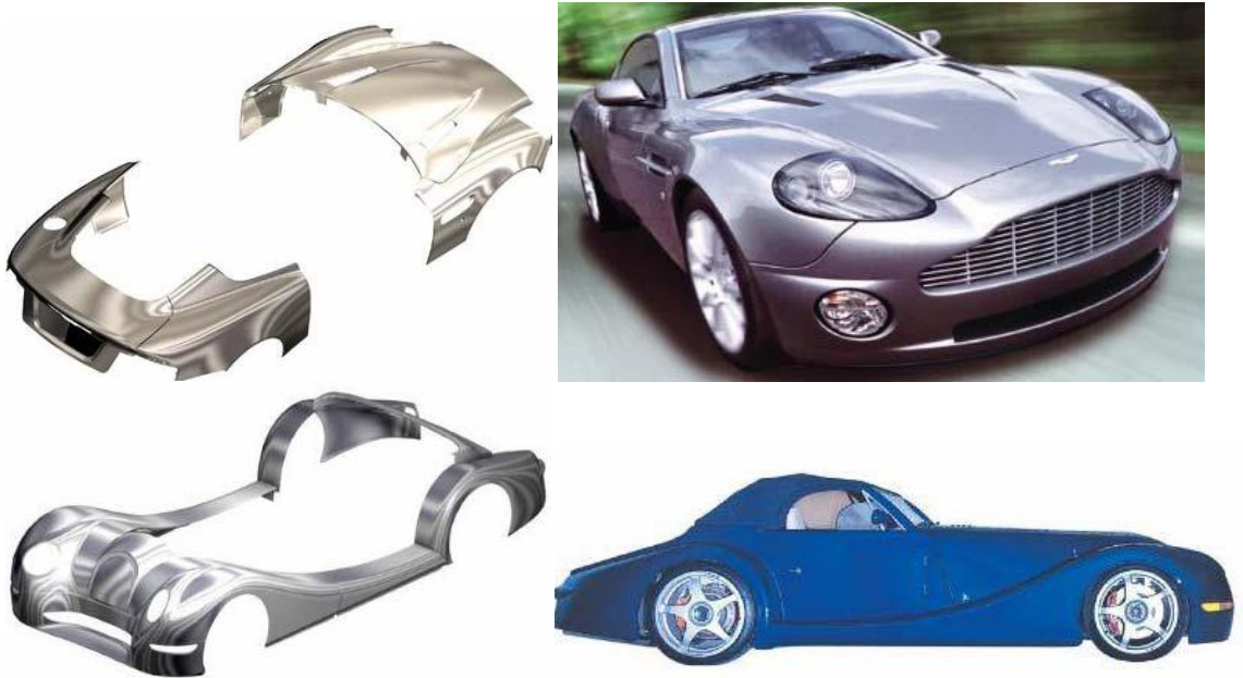
Figure 5 Superplastic forming used for automotive applications (a) Aston Martin Vanquish (b) Morgan Aero 8 (1)
