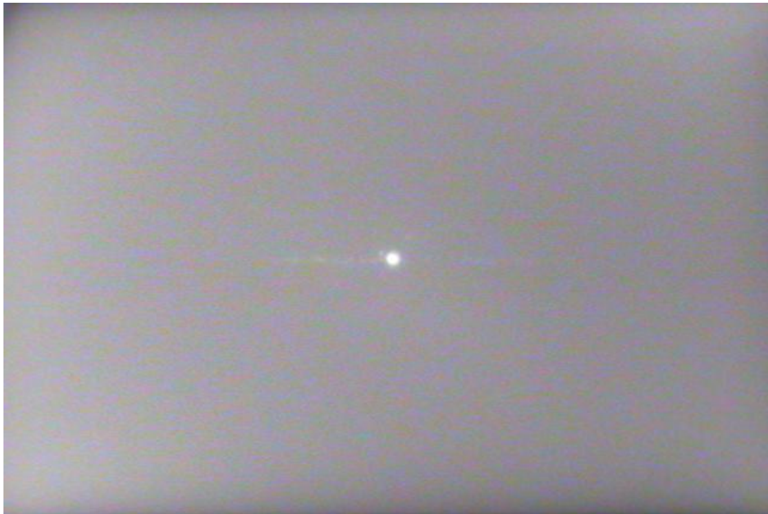
Figure 27 : Light through the waveguide as imaged on the IR camera.
