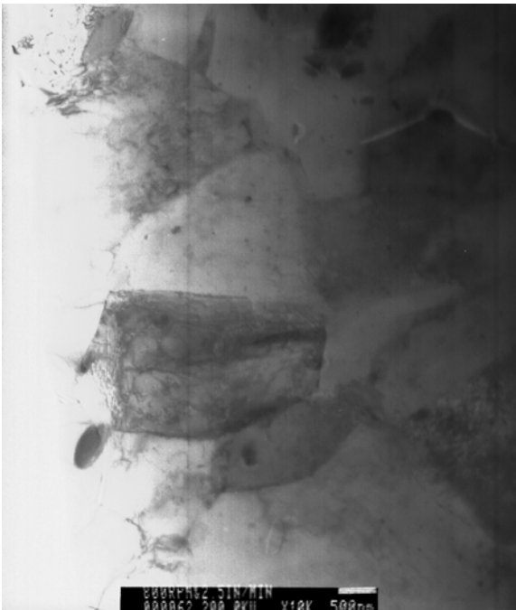
Figure 4-14 FS processed AA 5052 at 2.5in/min a) 400 rpm, b) 600 rpm, c) 800 rpm and d) 1000rpm
