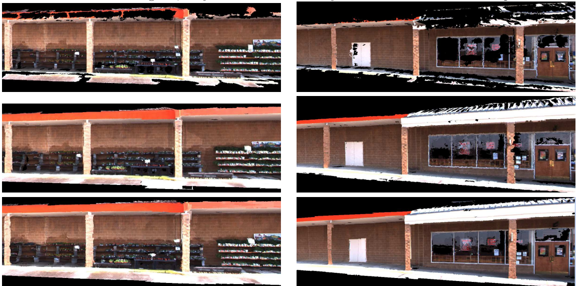
Figure 4.4: Visual comparison of depth maps associated with the 3D models shown below. From left to right: reference image, window-based stereo, plane-fitting stereo and BP-based plane-fitting. Notice how the depth estimates for the white textureless door are wrong in (b) and how that produces an incorrect surface in the corresponding 3D model below. Both (c) and (d) correctly handle the same door. Also notice that the very large depth errors found in the upper red and the bottom white textureless regions in (b) are discarded from the window-based 3D model since they otherwise would do much more harm than good, they are thresholded away based on the confidence map.
