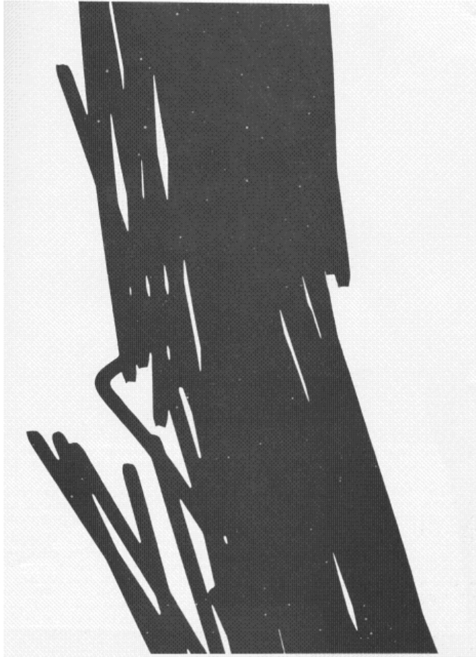
Figure 2-12 X-Ray Shadow Graph Showing Fracture of Individual Bead Wires Courtesy: Dynamics of Tire Failure
