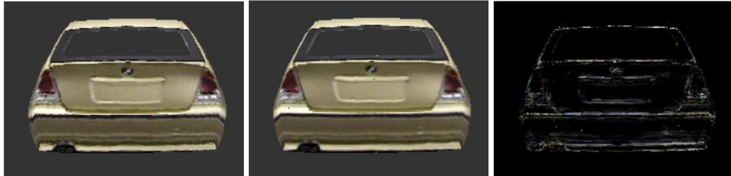
Figure 4.3: A side-by-side comparison of the BMW model rendered from a fixed view. (a) Rendering using traditional view-dependent texture mapping and an exemplar view. (b) Rendering from the same view using a Master Texture encoded image. (c) Direct image difference of first two renderings. Differences have been normalized to a range of 0-255 for visualization purposes. Only 5.6% of the 640x480 pixels in the image are different with a mean intensity difference of less than five.
