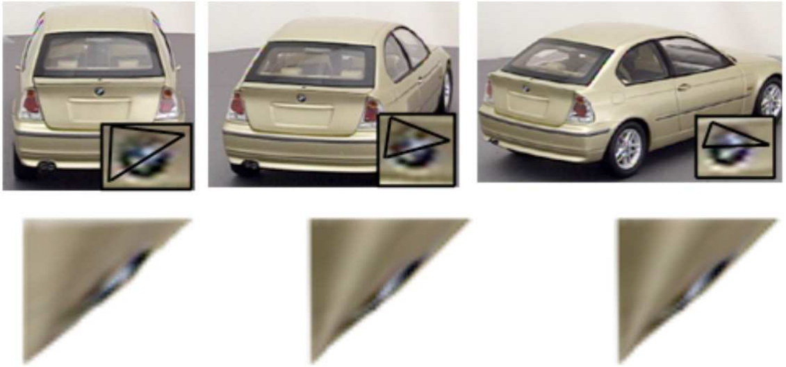
Figure 3.1: Example of facet parameterization. (top row) Three images of a real-world car object. A single mesh face corresponding (insert on each view, top row) as seen in each image. (bottom row) Facets are parameterized to uniform shape, size, and orientation.
