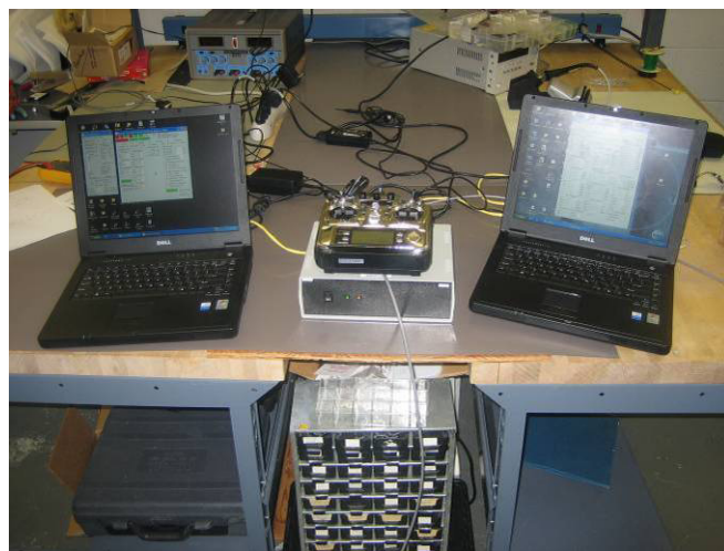
Figure 5.6 – Piccolo Ground Station Running a Simulation for Testing
