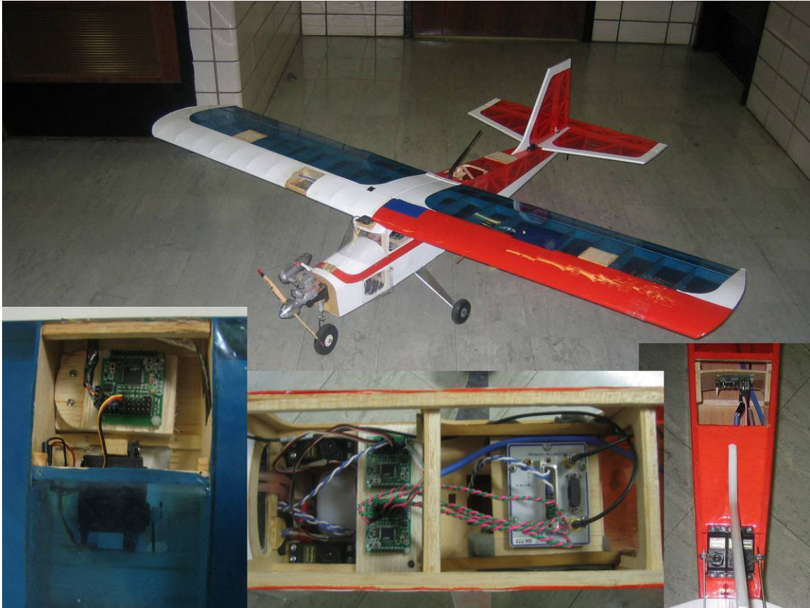
Figure 5.8 – In Aircraft Testing of Module and CAN Bus
