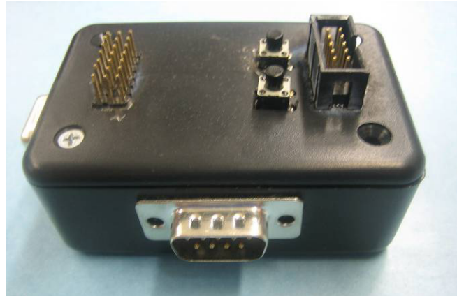
Figure 5.9 – Module Mounted in a Hobby Box
