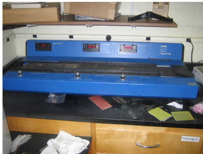
Figure 4.15 – ECE Department Solder Reflow Machine
