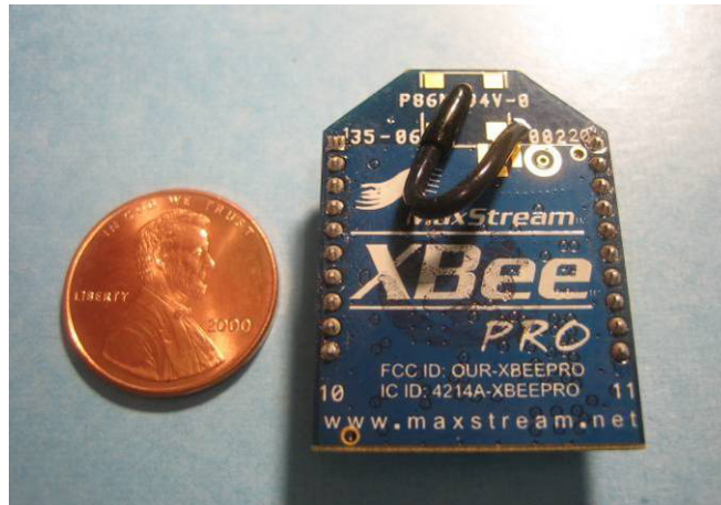
Figure 2.4 – MaxStream XBee-Pro Module
