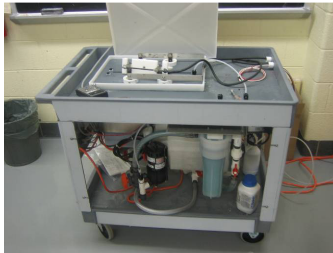
Figure 4.13 – ECE Department Through Hole Plating Bath
