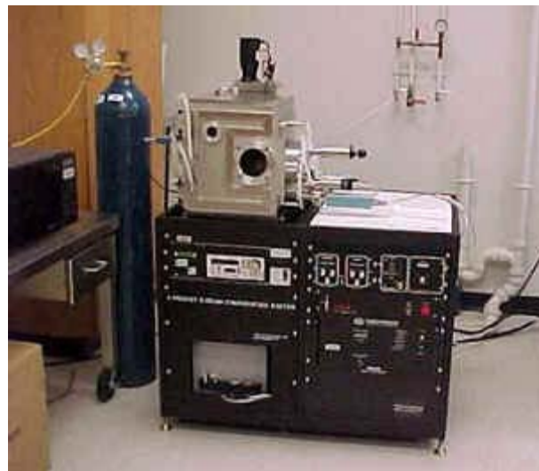
Figure 3.2.1 Electron-beam evaporator (University of Kentucky)
