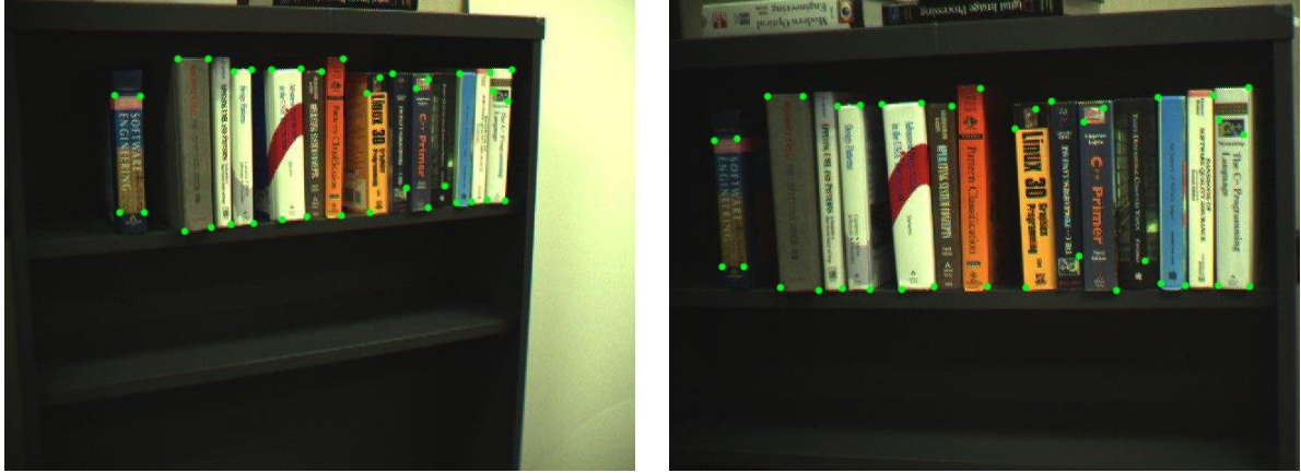
Figure 2.6: Show the point correspondences for the left and right views respectively which is used for obtaining the collineation between cameras
