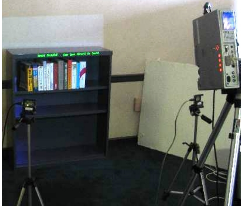
Figure 2.1: System setup with two cameras and a projector
