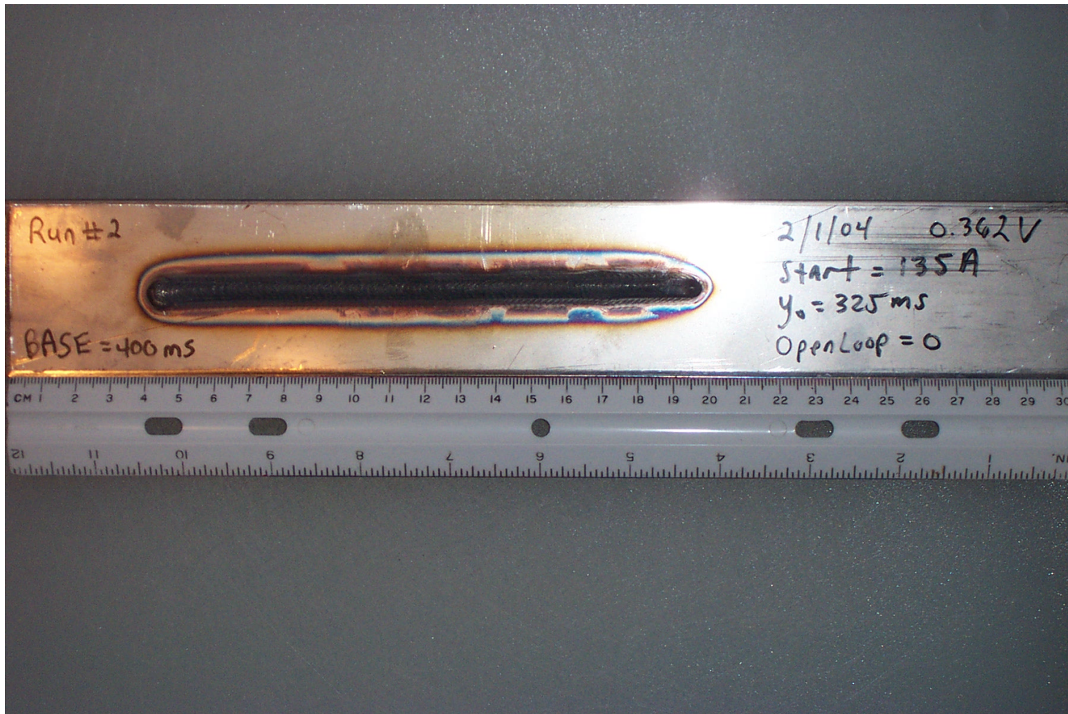
Figure 10-5 Topside Work Piece, Peak Time ref = 325 ms, Base Time = 400 ms, Start Peak Current = 135 A
