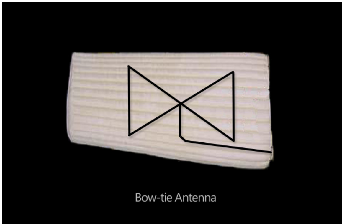
Figure 3.5: A Bow-tie antenna as mounted with a wing for UAV.
