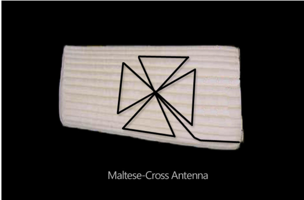
Figure 3.8: A Maltese-cross antenna mounted with a wing.
