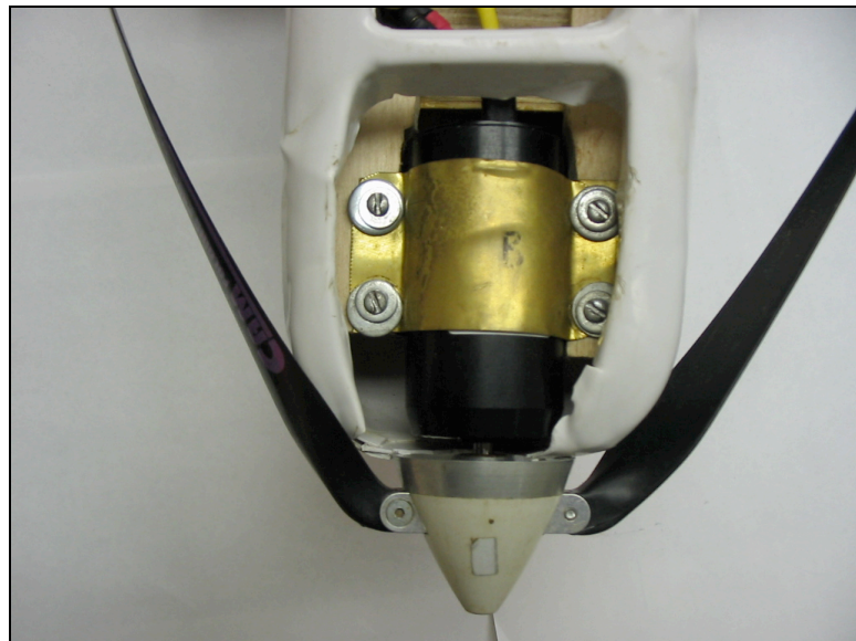
Figure 2.17: Motor, mounted in front of fuselage and held in place with thin brass straps.
