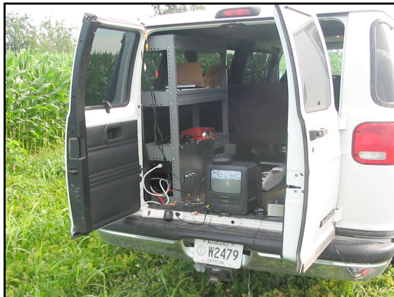
Figure 3.12: Ground Station, receiving live video stream transmitted from UAV. At the ground station, the live video feed was received through a receiver supplied with the video transmitter and recorded onto VHS video cassettes. Thus, the system
