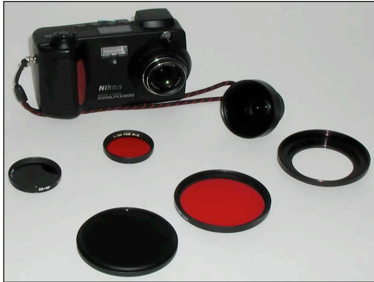
Figure 3.13: Nikon Coolpix 800 digital camera with additional filters.
