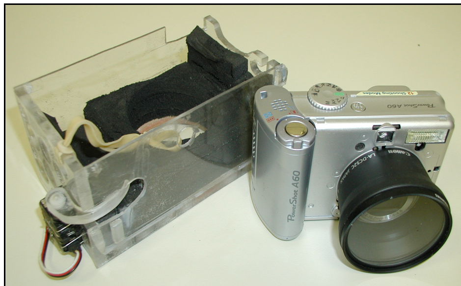
Figure 2.18: Digital Camera and Protective LEXAN® case
