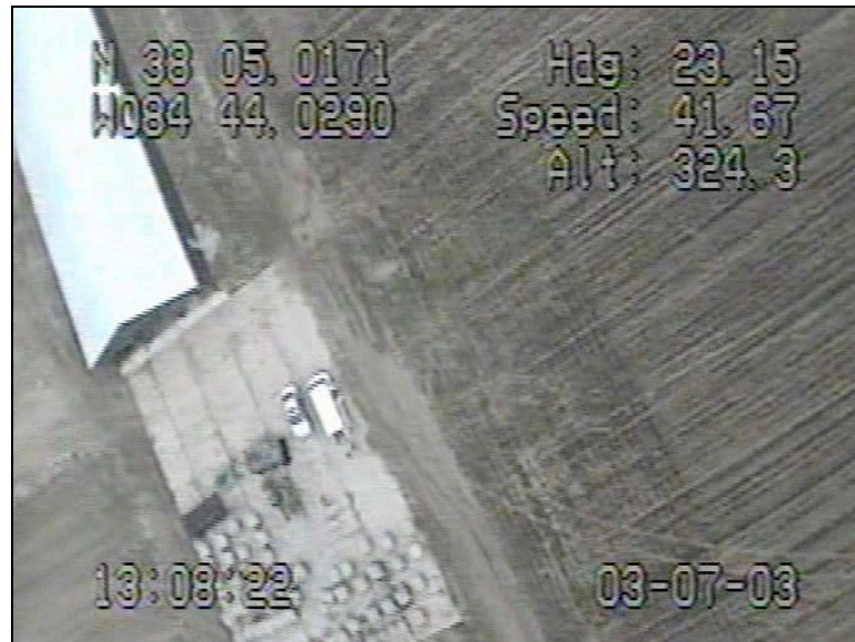
Figure 3.15: GPS data superimposed on images sent to ground station.
