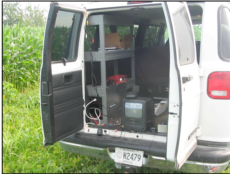
Figure 3.16: Ground Station with power supplies, TV, receiver, and other equipment.
