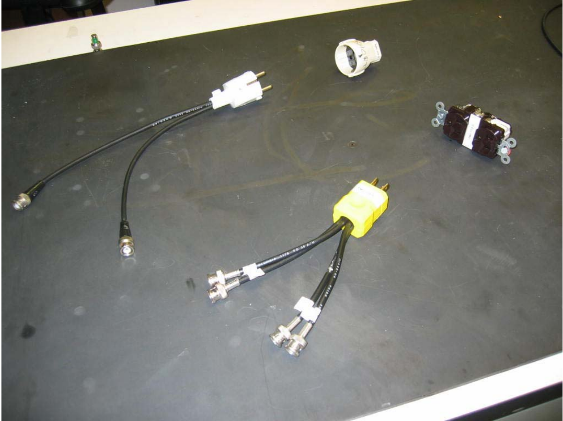
Figure 3.10: “T” EUT plug with ideally short leads on LISN side, and fixture compensation standards using EUT receptacle geometry
