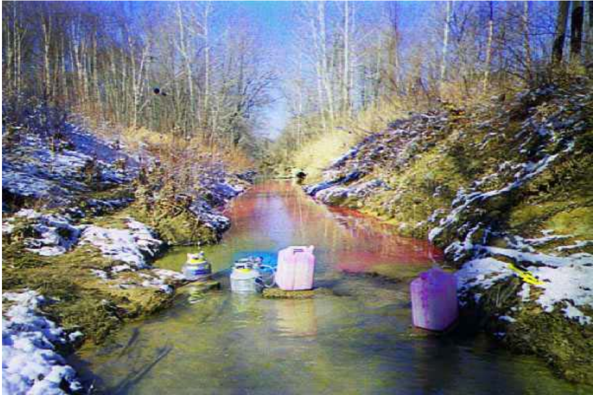
Figure 2.3:Tracer test in January 2002. The tracer plume produced by the slug injection caused the red coloration of the stream. The two carboys for slug injection and the propane tanks are visible at the injection point in the foreground. Looking downstream (north) from LBC-4.
