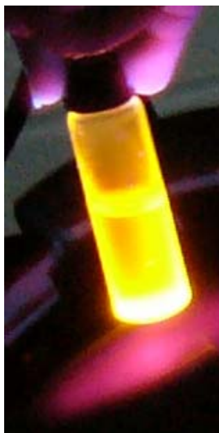
Figure 4. 11 Phosphorescence of (a.) film (b.) solution under the influence of a 365nm light source.
