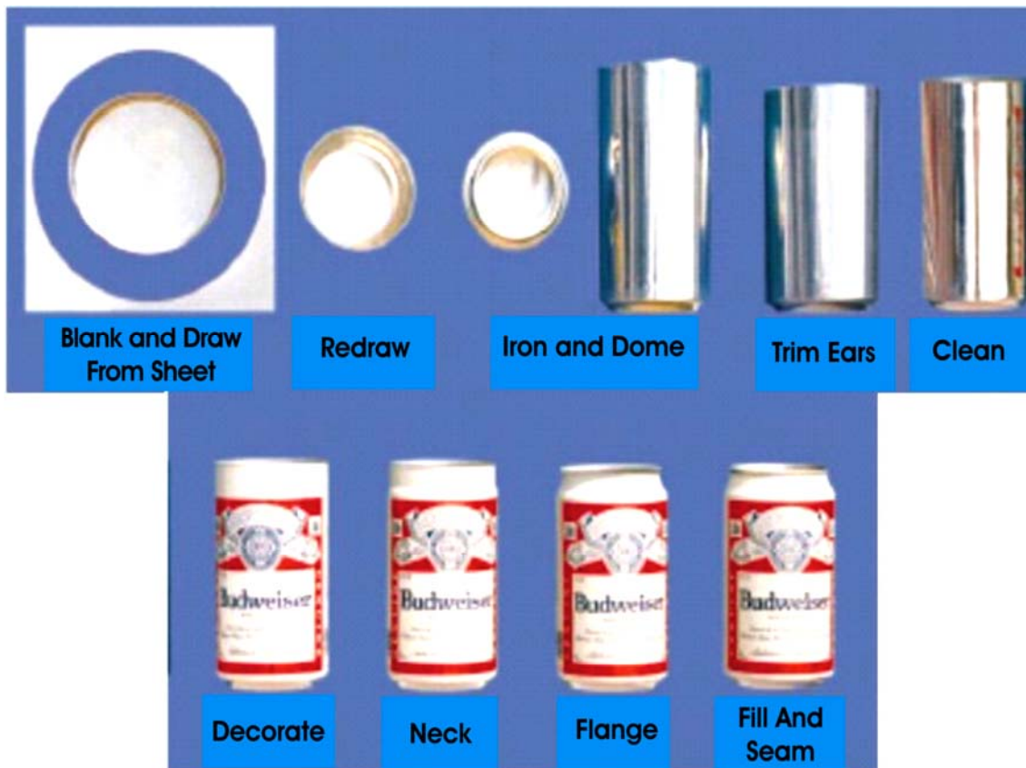
Figure 2.11: Transformation of Aluminum Beverage Cans During Manufacture
