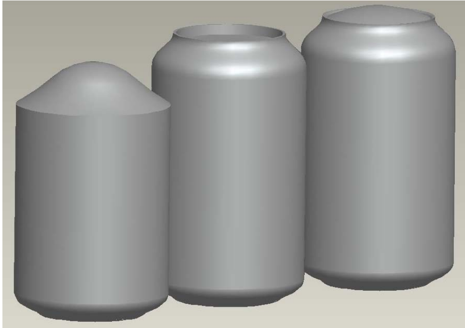
Figure 5.1: Aluminum Beverage Can Design (From left: Initial new inspiration, Current aluminum beverage can, Final New Unialloy Aluminum Beverage Can)
