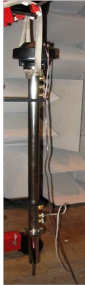
Figure 5.14 Vertical impedance tube measurement setup.
