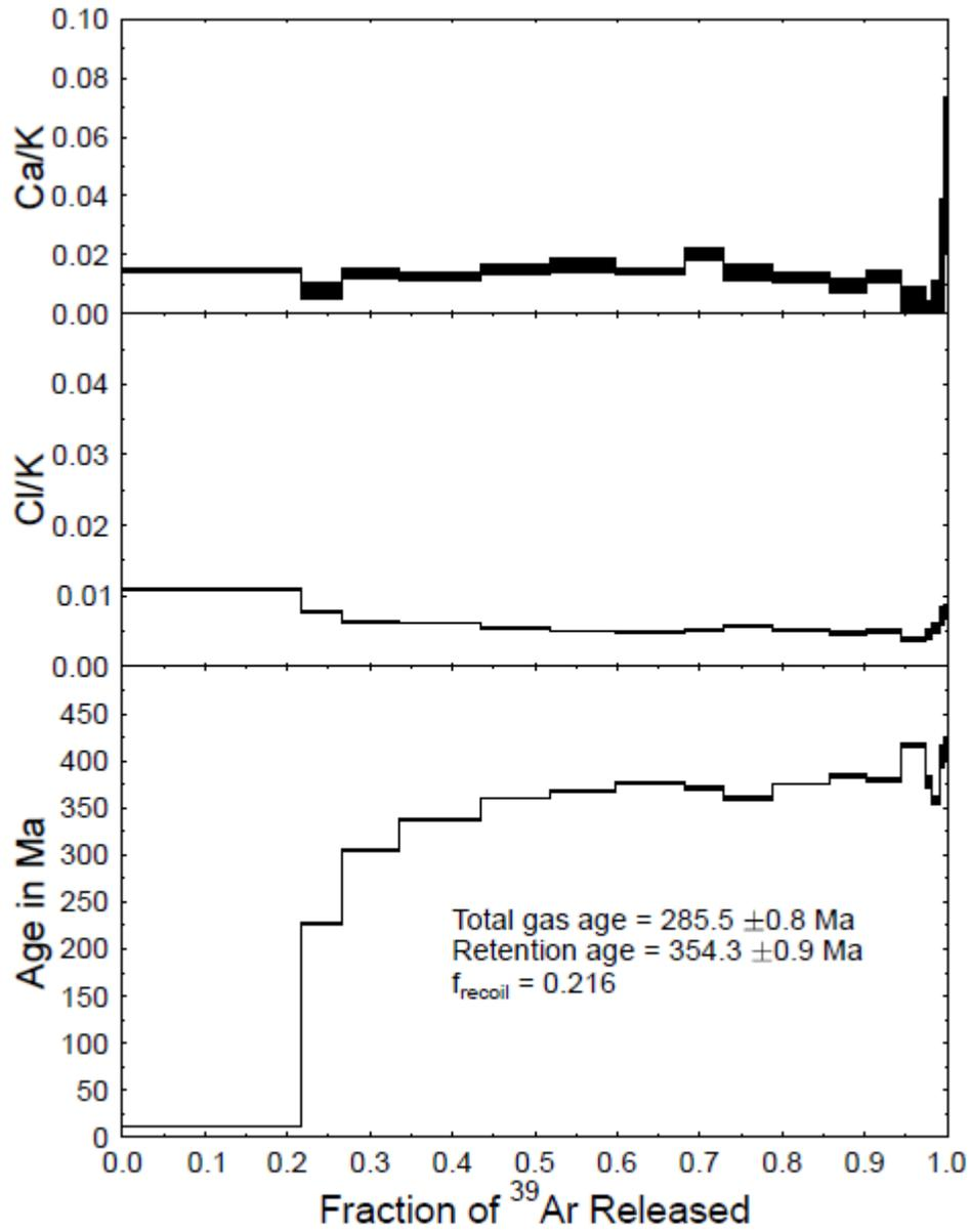
Figure FA51 – Ar-Ar spectrum for the sample BP-1.
