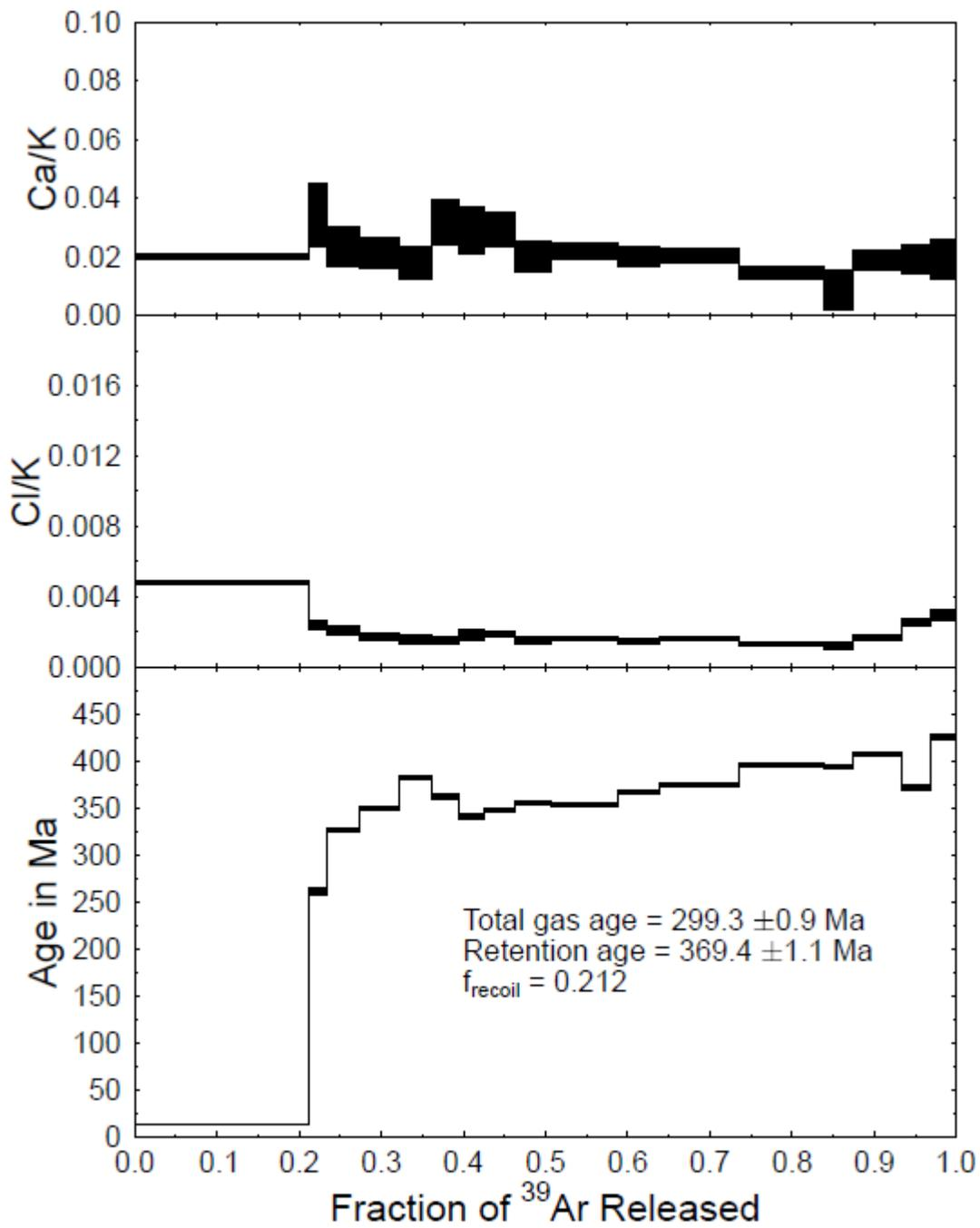
Figure FA48 – Ar-Ar spectrum for the sample OH3-1
