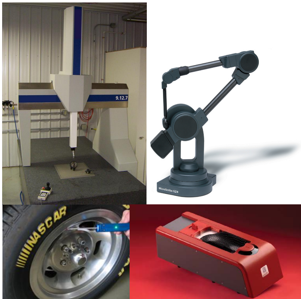
Figure 1.2, Examples of contact scanners [21-24]
