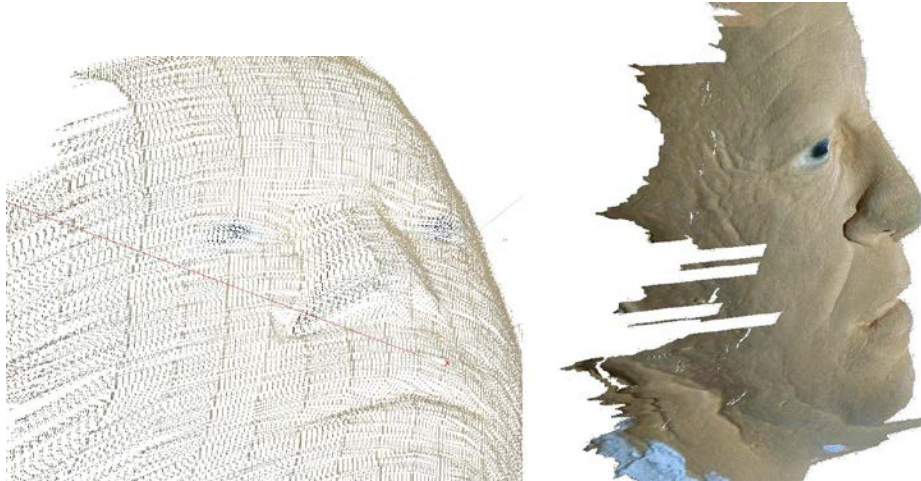
Figure 1.17, MCP scan of a latex bust, (left) MCP data points with interpolated linear fill regions, (right) result after smoothing and other post-processing steps
