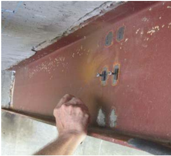
(a) Attaching tabs for gages
