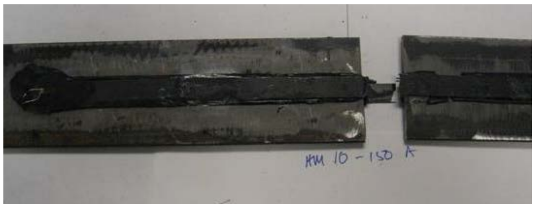
Fig. 2.14: Typical CFRP delamination seen in ultra high modulus CFRP
