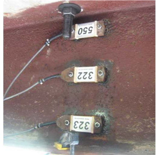
(b) Attached reusable strain gages
