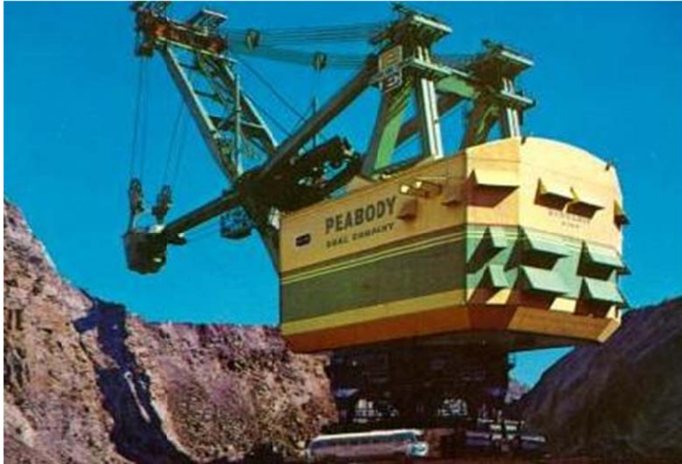
Figure 6.5: c. 1964 Peabody Coal Company (from www.muhlenbergcountyky.com , but also at Duncan Cultural Center) Machinery used to extract overburden in surface mining operations
