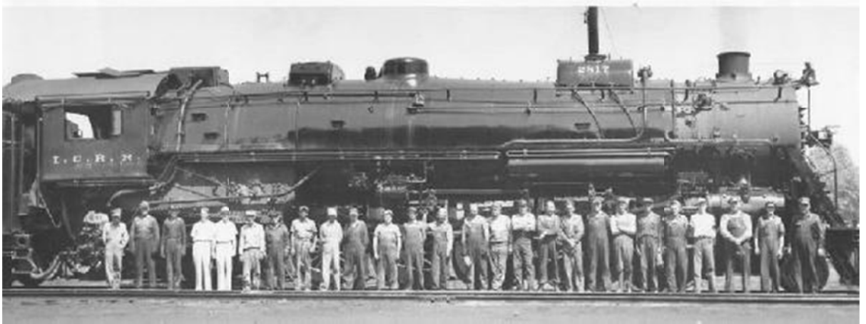
Figure 6.4: “Mountain type Locomotive would haul 100 coal cars from Central City to Paducah for further distribution circa 1955” (from www.muhenbergcountyky.com )
