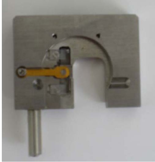
Figure 3-17: Bottom side of a tip holder for vapor measurements. The gold piece holds the cantilever.
