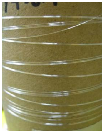
Figure 4.10. High luster of dry-jet spun fiber
