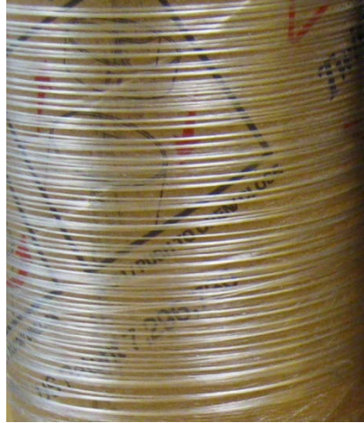
Figure 4.4. Wet-jet spun fiber stretched at 107 °C
