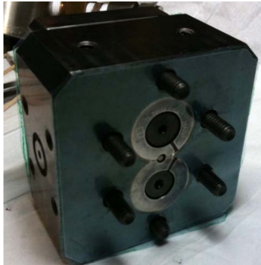
Figure 2.5. One mil fluoropolymer gaskets to increase side clearance
