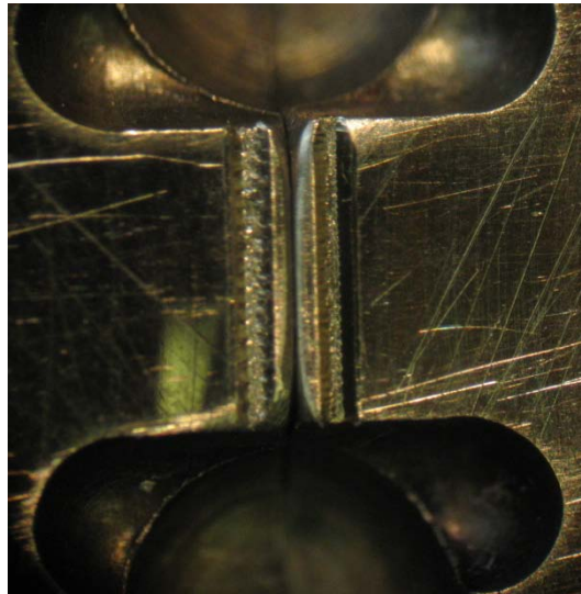
Figure 2.7. Bearings machined with channels
