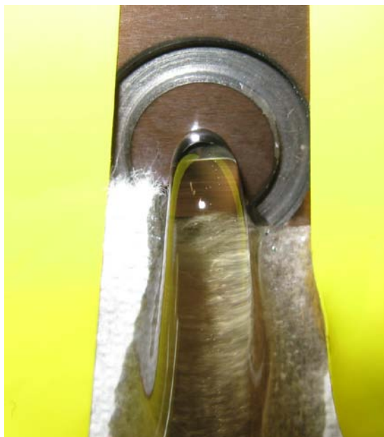
Figure 2.9. Dope flow without bubbles
