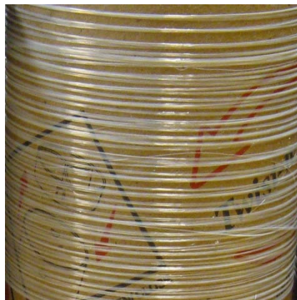
Figure 4.6. Dry-jet spun fiber stretched at 110 °C
