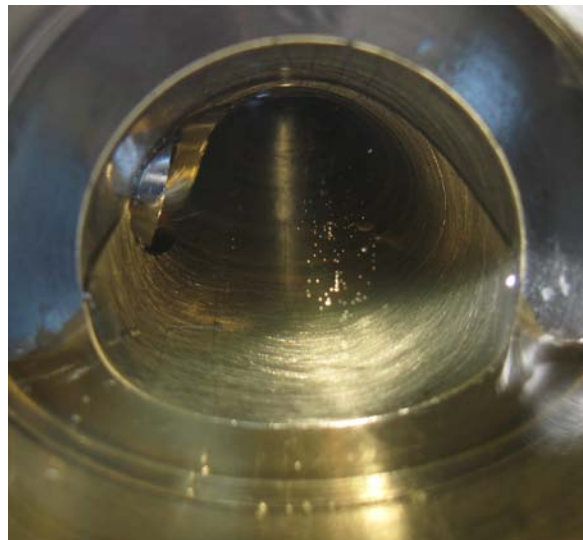
Figure 2.6. Resulting decrease in bubbles due to addition of gaskets
