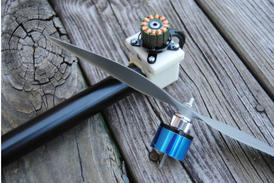
Figure 34: Brushless Outrunner Motor
