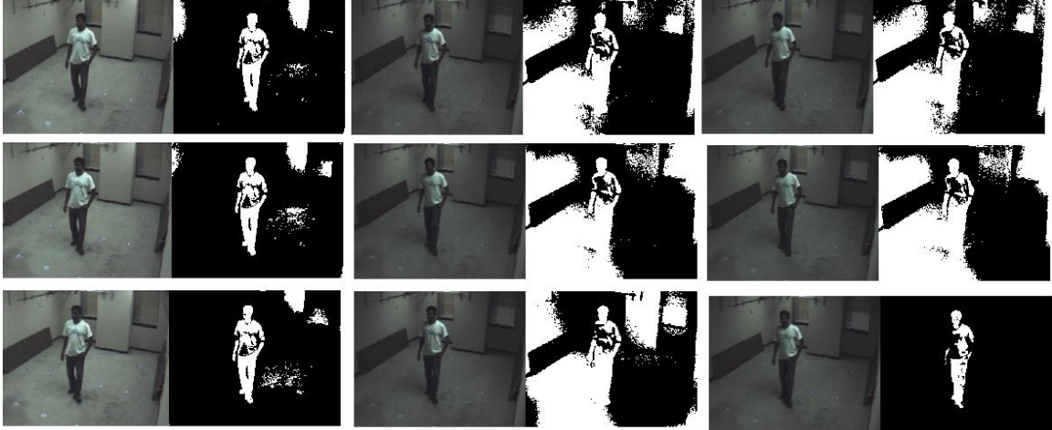
Figure 5.3: Illustration of illumination compensation from high to low : a) The first column shows the frame before the illumination change for 2 nd , 3 rd and 4 th . b) The second column shows the actual illumination change. c) The third column shows the compensation by 2 nd , 3 rd and 4 th .
