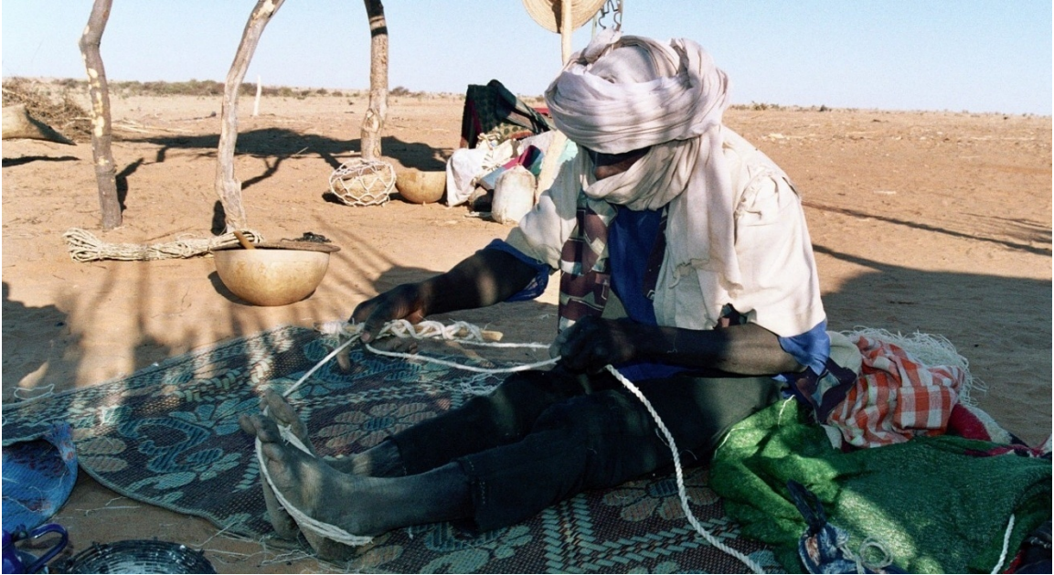
Figure 9.7: (Photo, above, ceeḍu 2007) The man twines the cords he has twisted into a rope.
