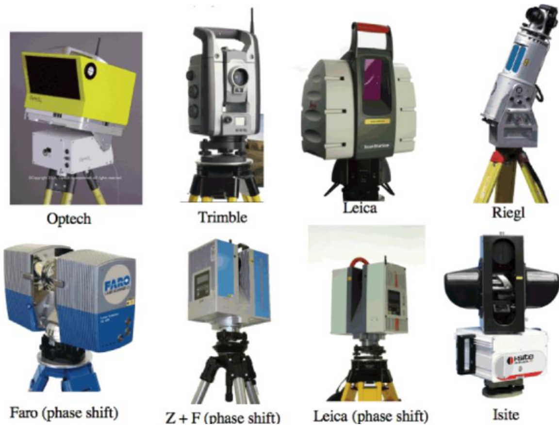
Figure 1.1: Ground-based LiDAR scanners (time-of-flight unless noted as otherwise) [8, 9, 10, 11, 12, 13, 14, 15, 16].
