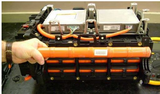
Figure 3.9: Honda Insight battery pack [59]
