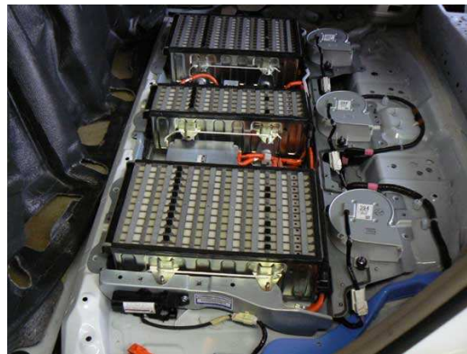
Figure 3.7: Toyota Highlander battery pack [59]
