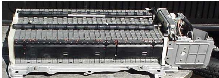
Figure 3.5: Toyota Prius battery pack [59]
