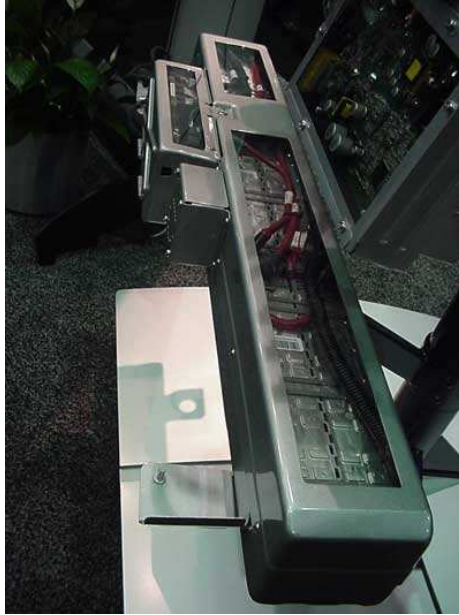
Figure 3.10: Saturn Vue battery pack [59]
