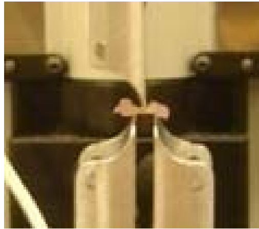
Figure 3.3.5a: 3-point bend test to failure to assess structural properties [7]
