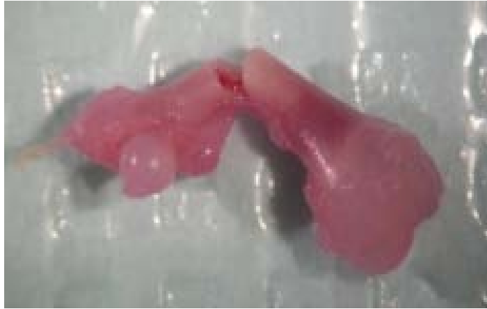
Figure 3.3.5b: Image of femur post 3-point bend test to failure showing the fracture through the bone shaft
