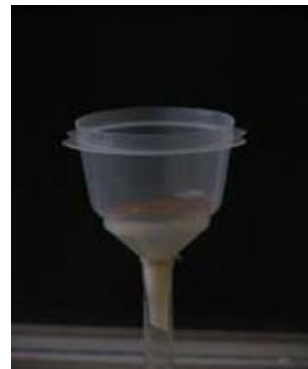
Figure 2.2: Different devices to measure wetting rate. a) Tension table; b) Drop former; c) Splash-guard cup with a mesh to provide free drainage.
